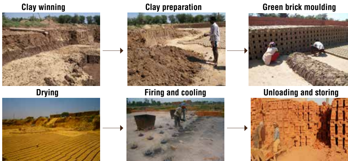
Figure 1: Brick making process
